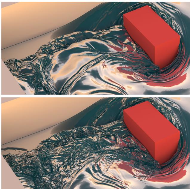
Fig. 6: **Top:** Without *frozen core* extension and improved advection from §3.6. **Bottom:** Same frame, with modifications from §3.6. Note that the turbulent wake behind the block is lost entirely without our improvements.
