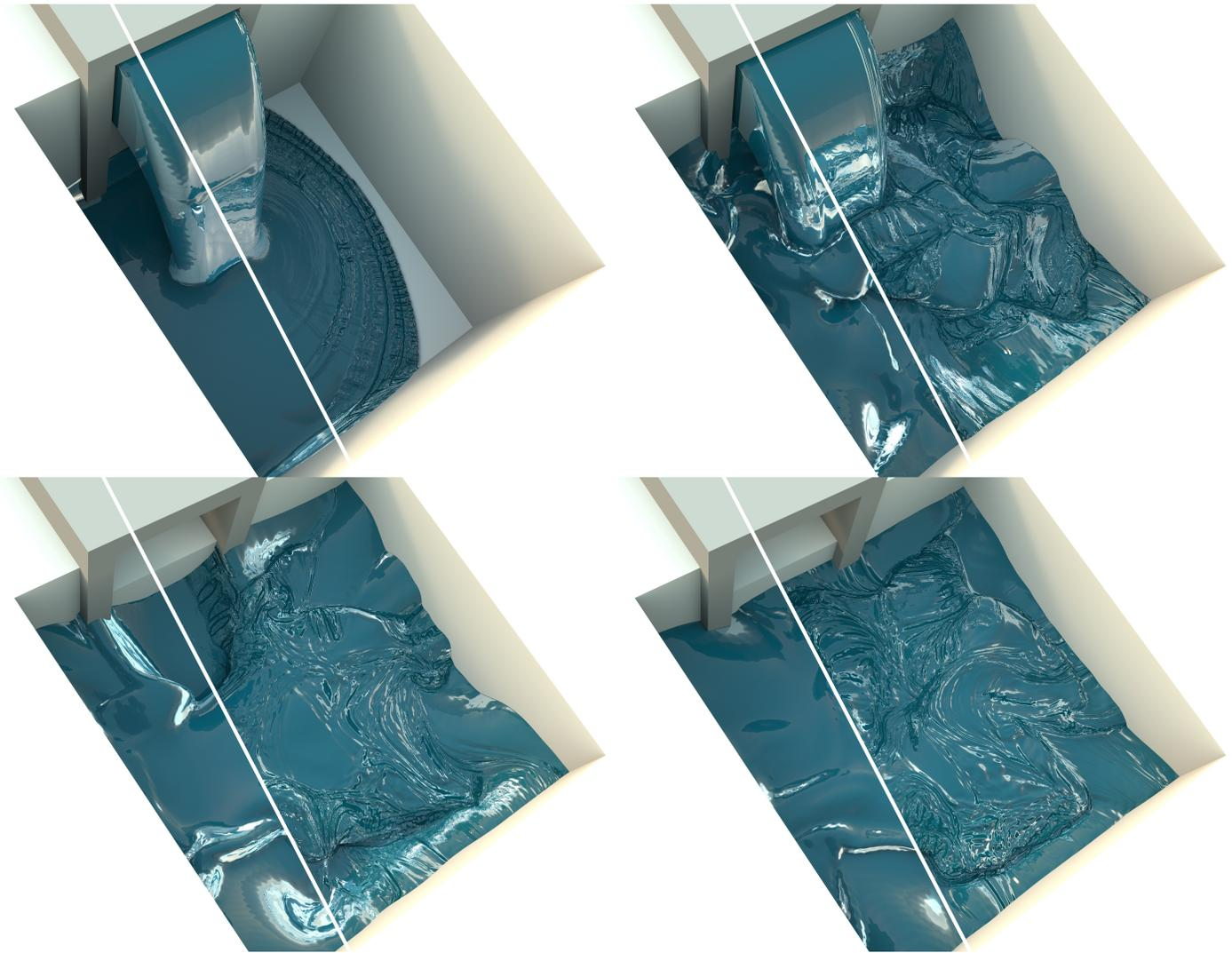
Fig. 8: A  $100^3$  PhysBAM simulation, up-resed to  $800^3$ . The left half of each image shows the original simulation, and the right shows our up-resed version. The  $8\times$  up-resing only took approximately twice the time of the original simulation.
