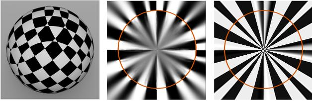
Fig. 3: Left to right: a sphere with a checkerboard surface; the center slice of the sphere’s extension field, computed using fast marching; the same slice computed using our *Nacelle* variant. Our variant is faster and does not smear out the scalars. Computing the  $200^3$  extension field took 3 minutes and 20 seconds with fast marching, and 21 single-threaded seconds with our algorithm.
