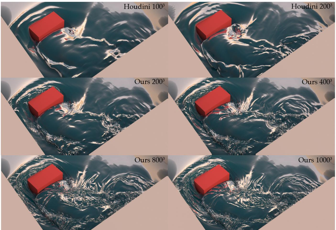
Fig. 10: **In reading order:** Original  $100^3$  Houdini simulation, 2, 4, 8, and  $10\times$  upres, and direct  $200^3$  Houdini simulation. Note how even at  $2\times$  upres, higher frequency waves than those in the direct  $200^3$  solution are captured.
