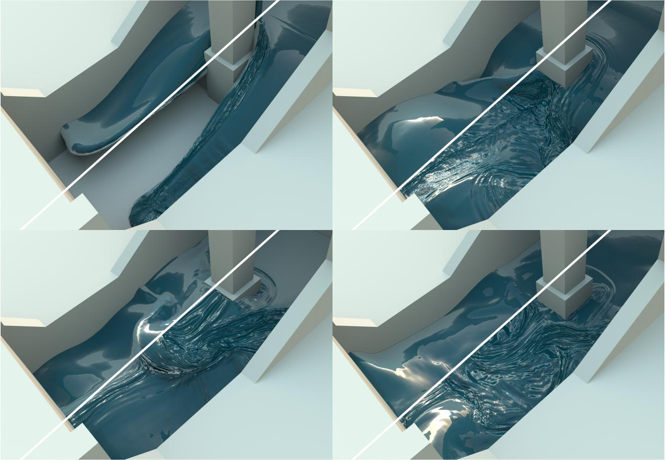
Fig. 7: A  $100^2 \times 50$  PhysBAM simulation, up-resed to  $800^2 \times 400$ . The left half of each image shows the original simulation, and the right shows our up-resed version. Our simulation took roughly  $10\times$  the time of the original, whereas a brute force simulation would take roughly  $512\times$ , i.e.  $8^3$ , the time. The source and height values around the column were clamped to zero as respectively described in §3.7 and §4.
