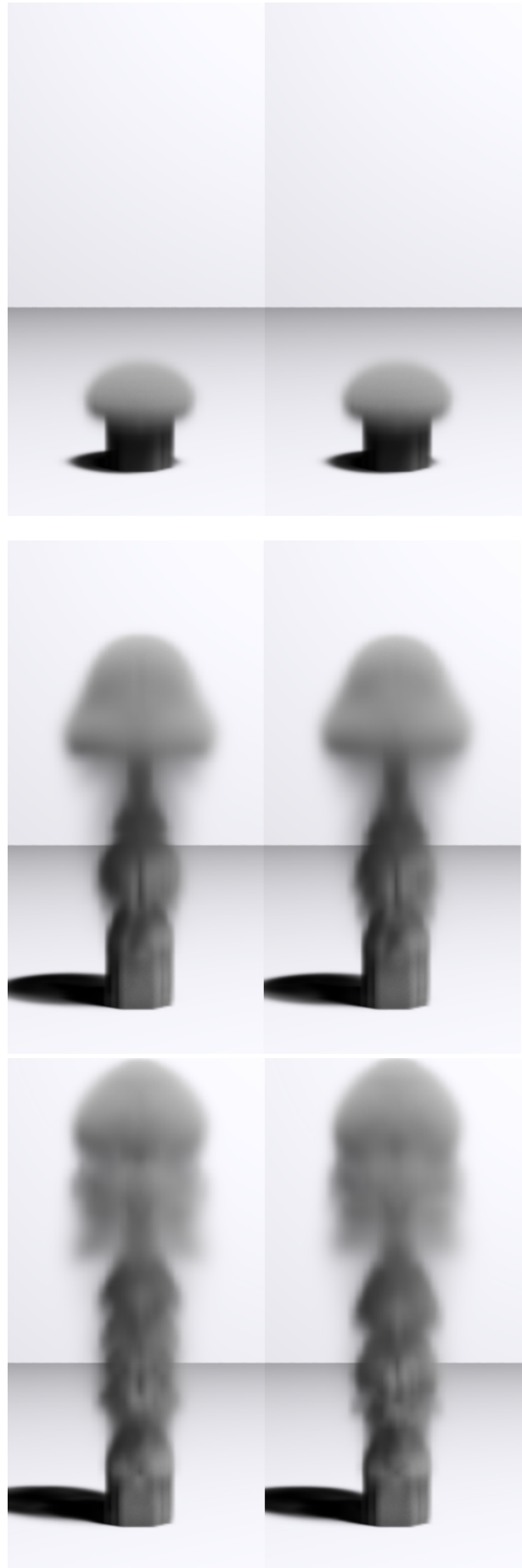
Figure 5: 3D Smoke rising with standard Jacobi (left) and Mehrstellen Jacobi (right). The results are virtually identical, but the pressure solve runs 33%.
